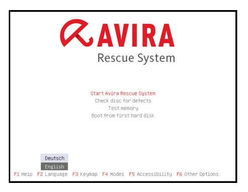
The Welcome area of the Avira Rescue System explains the three scan and repair functions of the Wizard. The Avira Rescue System will not delete infected files but renames detections to *.rend* files, in order to make them still accessible.
